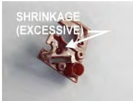
Figure 28-1 Shrinkage (excessive).
