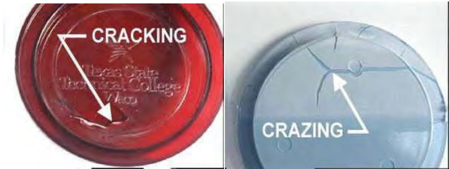
Figure 19-1 Cracking and crazing.
