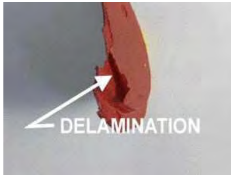
Figure 20-1 Delamination.
